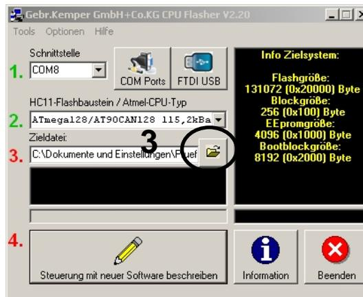
7. Pos .4 Flash the controller with the new software
